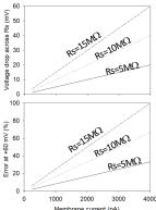
The calculated voltage drop across the series resistance as a function of the membrane current.
