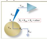
Series resistance is the sum of all of the resistances between the input of the patch clamp amplifier (blue triangle) and the cell membrane. It is the sum of the pipette resistance (R<sub>pip</sub>), any access resistance, R<sub>a</sub> and other forms of resistance located between the pipette tip and the interior of the cell.
